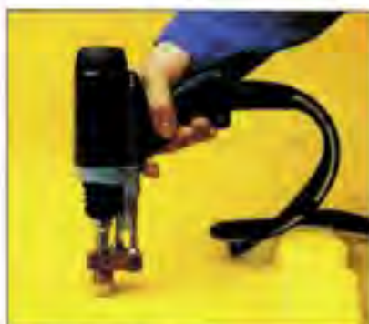
Place welding gun pull trigger — finished
