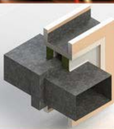
Dampened Duct through Intubatt 1
