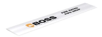
BOSS FR Pipe Wraps are intumescent composition-based elastomeric thermoplastic polymers, designed to provide high volume expansion and pressure sealing around PVC pipes and insulated metal pipes. Tested systems includes PVC, Polypropylene, MDPE, HDPE, HPPE and ABS up to a size of 200mm diameter pipes through concrete / blockwork floors and walls as well as light weight partitions.
