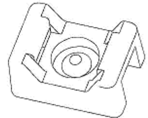
As installed after extension is broken off
