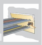
Transfer measurements onto mineral wool panel, but add about 3 mm on height and width of panel cut (this will result in a tighter fit). Now cut panel into as many pieces as necessary to fit in the opening.
